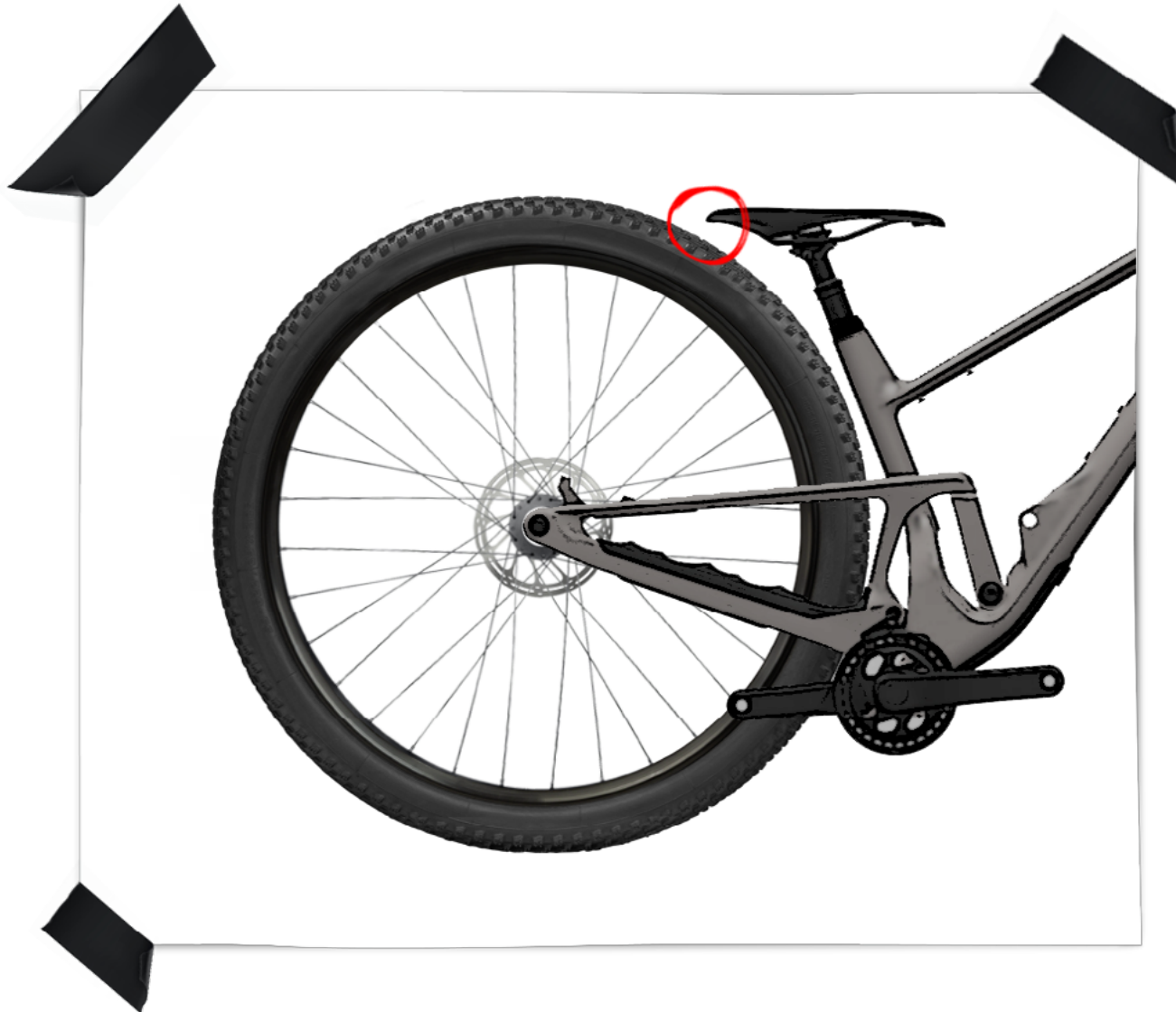
Fig.4 – saddle clearance at full compression
